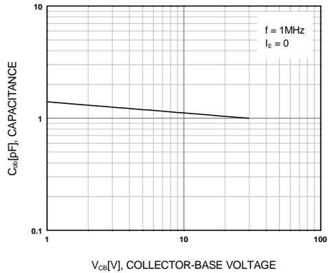
Figure 4. Output Capacitance
