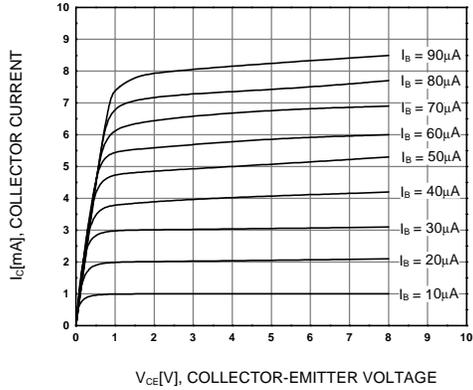
Figure 1. Static Characteristic
