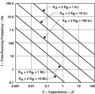
Figure 14. Free-Running Frequency
