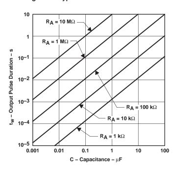
Figure 11. Output Pulse Duration vs Capacitance
