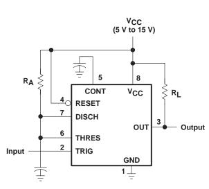
Pin numbers shown are for the D, JG, P, PS, and PW packages.
