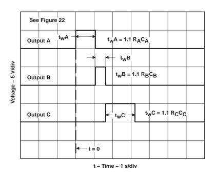
Figure 23. Sequential Timer Waveforms
