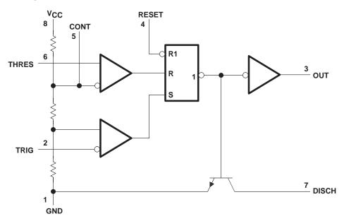
Pin numbers shown are for the D, JG, P, PS, and PW packages. NOTE A: RESET can override TRIG, which can override THRES.
