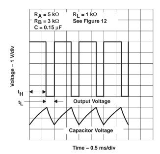
Figure 13. Typical Astable Waveforms
