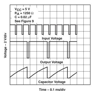
Figure 17. Divide-by-Three Circuit Waveforms
